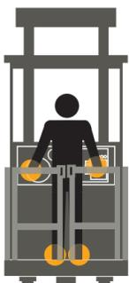
**Four points of solid contact on the SP 3500 Series,** with right-hand fixed control, enhance operator stability and confidence at height.
