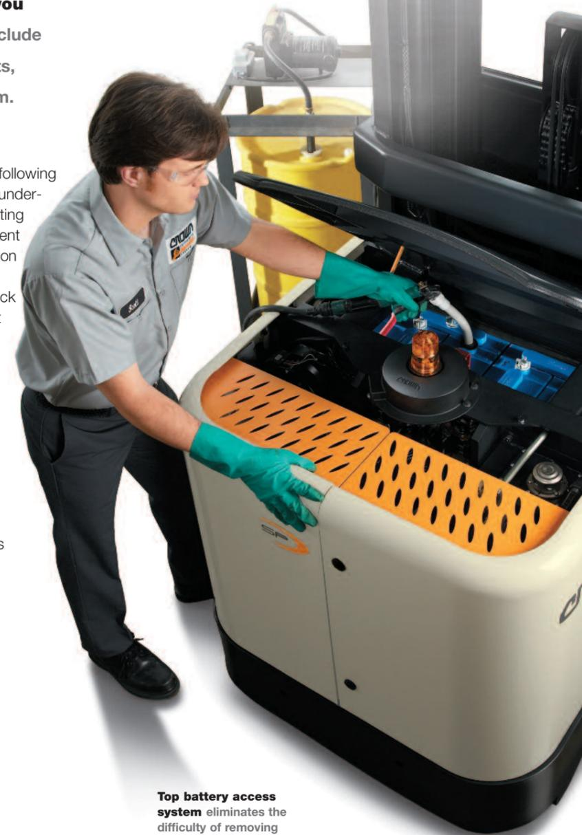
Top battery access system eliminates the difficulty of removing batteries to add water, check electrolyte levels, measure voltage and perform other routine maintenance.
